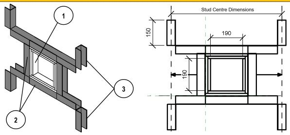
\*Note: Support legs are provided to fit to the specified stud centres. Stock centre sizes include: 400, 600 and 1200mm c/c.
