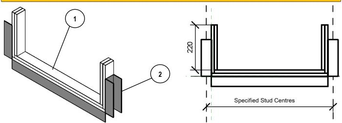
\*Note: Modular openings can be produced to be fixed directly to vertical studs as a single composite member without the need for additional support legs. If more flexible opening dimensions are required then adjustable openings should be selected.
